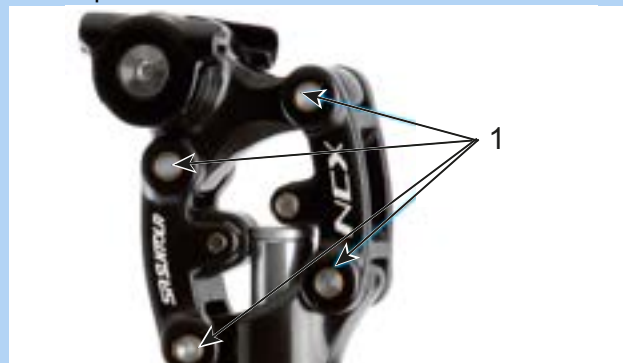
Figure 149: SR Suntour suspension seat post lubrication points
