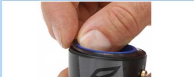
Figure 193: Detaching the seal lip ring
