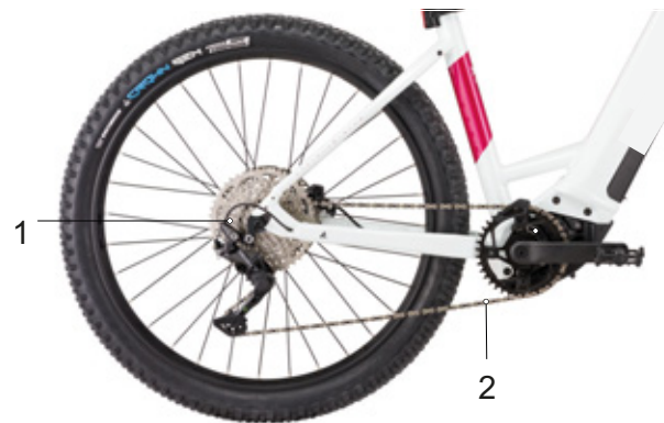
Figure 26: Chain drive with derailleur gears
