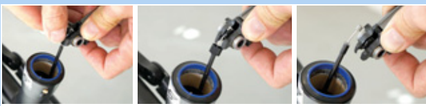
Figure 191: Removing the Bowden cable
