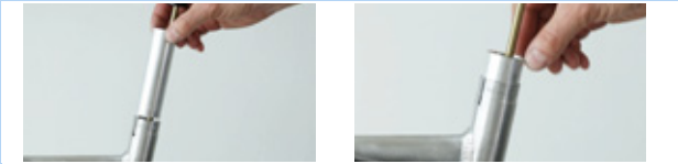
Figure 181: Inserting the slide bushing tube into the seat tube
