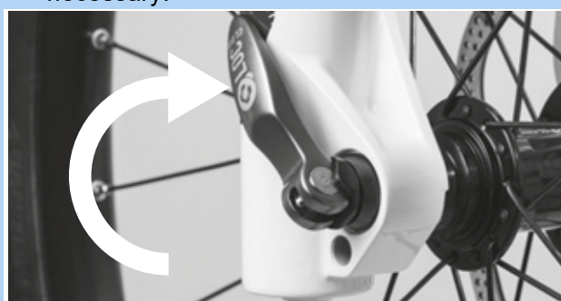
Figure 75: Closing the quick release
