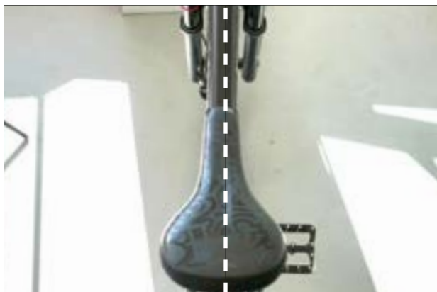
Figure 80: Positioning the saddle in direction of travel
