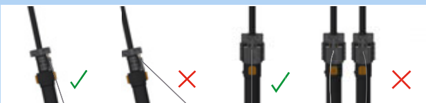
Figure 177: Correct and incorrect Bowden cable
