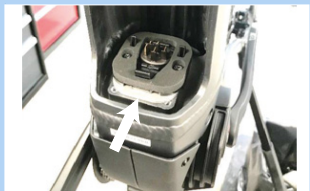
Figure 51: Fitted adapter plates
