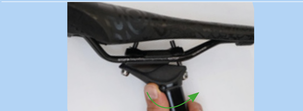
Figure 201: Opening the height adjustment
