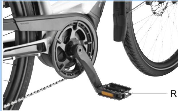
Figure 78: R-pedal in the right-hand crank arm
