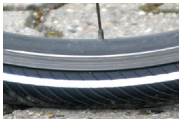
Figure 97: Correct tyre pressure. The tyre is barely deformed under the load of the body weight
