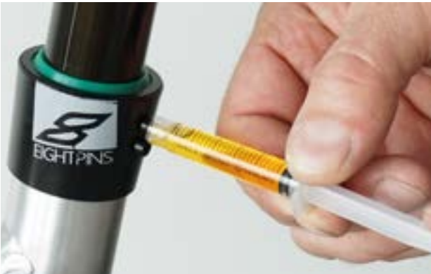
Figure 135: Lubricating the seat post tube
